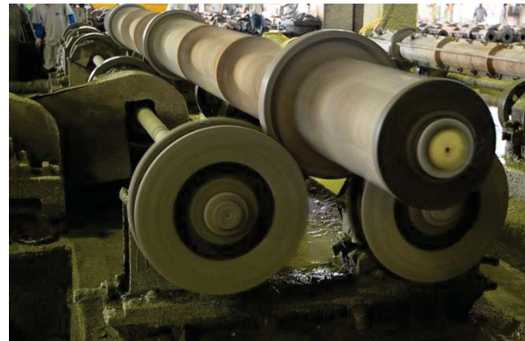
A mould being spun on one of our centrifugal spinning machines
