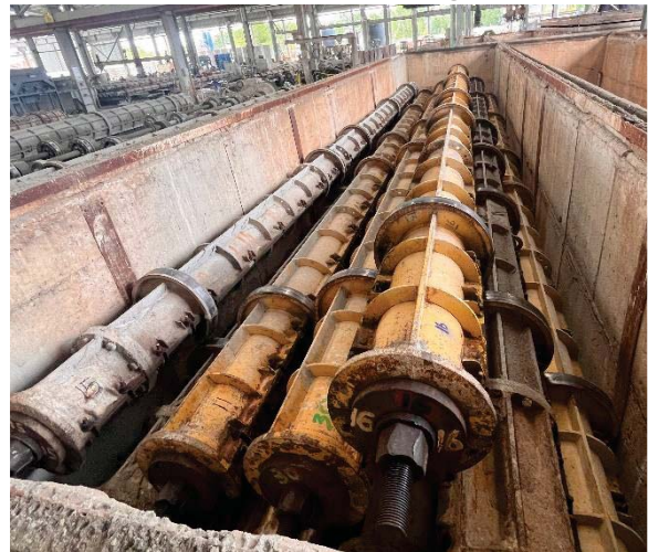
Moulds in one of our curing ovens
