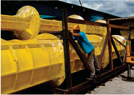
Left: Finished moulds for monopoles prior to shipment to a customer.
