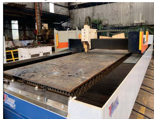
Cutting a steel plate for a mould
