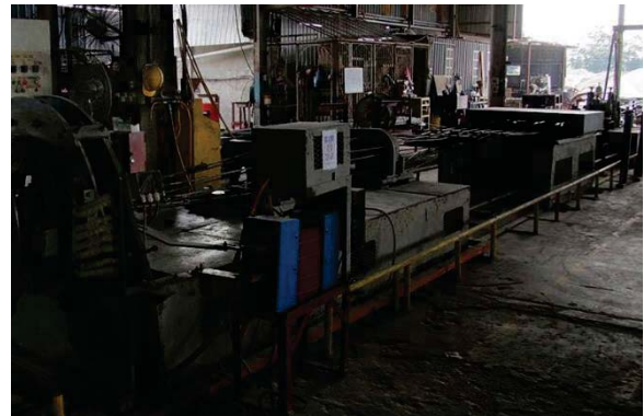
One of our automated steel caging machines
