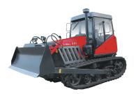
The walking device is a crawler type, mainly used for pulling and driving various supporting equipment, agricultural machinery for completing agricultural operations, earthwork operations and transportation operations. The Company's crawler tractor products have better soil adhesion, suitable for wet soil and soft ground.
