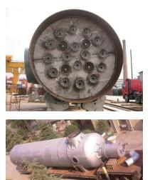
Burner for large CO incineration serves to mix supplementary fuel gas and combustion air and burn evenly.
