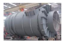
We developed a type of low pressure water sealed tank in 2011. When compared to previous model of water sealed tanks, our product can reduce pressure drop by more than 75% during the transportation of low-pressure gas phase medium with large flow and large flow channel, achieving good energy saving effect.
