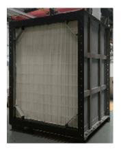
The product's core is made of modified polymer plates and the shell is made of metal with anti-corrosion coating. It is mostly used in flue gas de-whitening projects. Compared with material such as metal and glass, plate form polymer phase transition agglomerator is compact and lightweight, and is resistance to acidic corrosion of sulfur and nitrogencontaining compounds.
