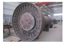
Waste heat boiler is a fire tube boiler connected to heat
