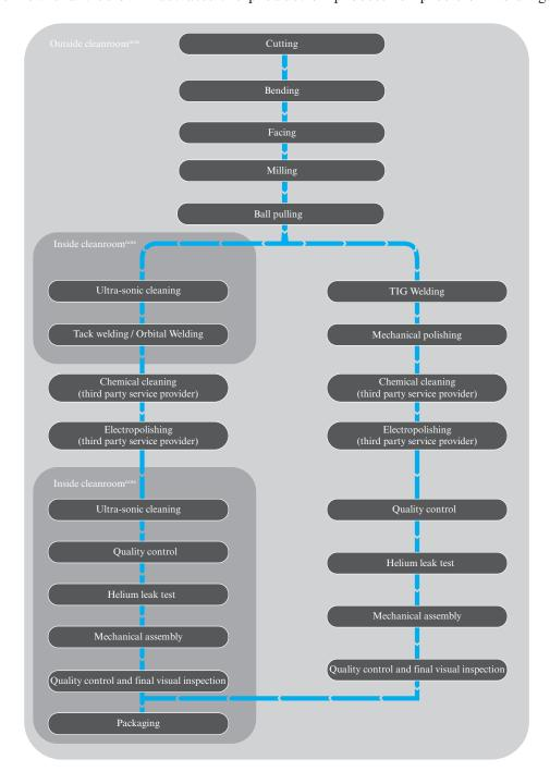
*Note:* Depending on the type of products for precision welding and customers' requirements, certain products which require high purity welds such as gas lines are processed in a cleanroom. For other products, all steps are conducted outside the cleanroom except for packaging.
