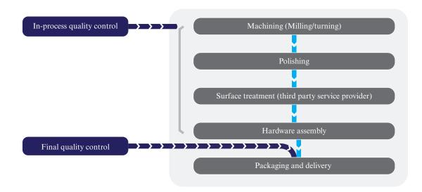
Depending on the complexity of the product specification, the project lead time for precision machining from receipt of purchase orders to delivery normally takes around 4 to 17 weeks. The production process consists of the following steps:
