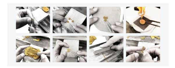
• Carving (鏨刻). Carving involves fixing the workpiece on a rubber plate by using various carving tools, striking the chisel with a hammer, and carving various patterns on the surface of the gold through diverse carving techniques.
