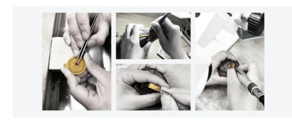
• Heat treatment of enamels (燒藍). The technique of heat treatment of enamels is a decorative process that entails the application of colored enamel glaze onto the surface of gold products, which results in a vibrant and multi-hued appearance.
