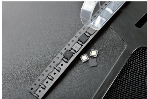
Carrier tape with width of 16mm containing our MEMS and sensor packaging product for illustration purpose
