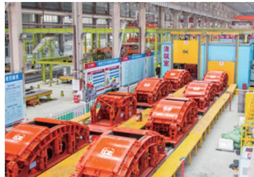
*Our PC component carousel production line (tunnel segments)<sup>(Note)</sup>*
