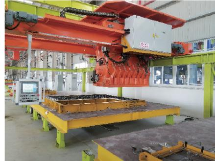
*Our PC component carousel production line (other construction components)*
