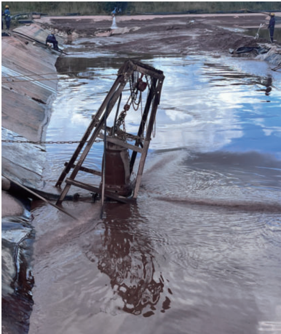
Kinsenda礦場水倉機械化清泥 Mechanized Mud Cleaning in Water Tanks at Kinsenda Mine
