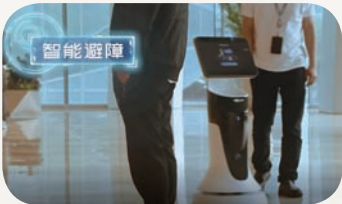
Tour guide robot uses voice instructions and touch panel to realise intelligent guidance to avoid obstacles
