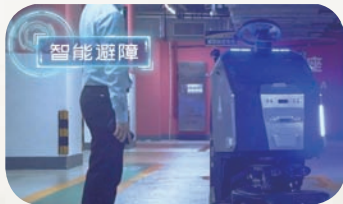
Cleaning robot self-completes charging, water supply and drainage circulation and efficiently executes floor washing task
