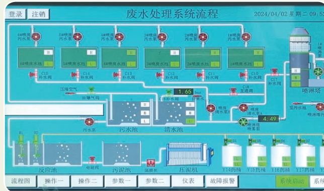
The changed wastewater treatment system flow 變更後的廢水處理系統流程
