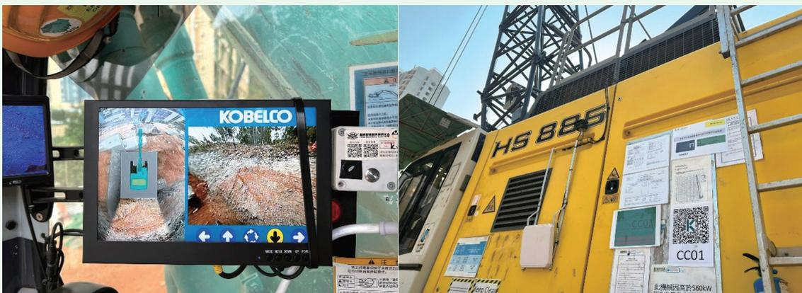
A 3D aerial-view with a full coverage of 360° around the machine is displayed
