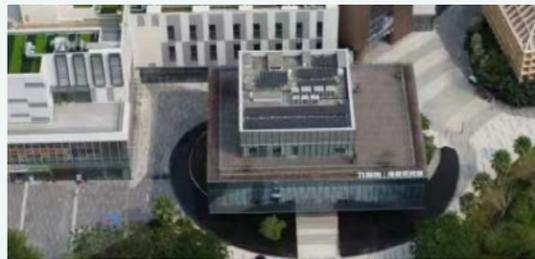
Tianjin Jinmao Place has installed photovoltaic galleries in the West Square, with solar photovoltaic panels mounted on top. It has an annual power generation capacity of 80,000 kWh, which can reduce carbon dioxide emissions by 76.8 tonnes every year.
