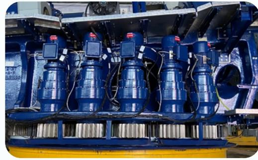
"New Generation of Yaw Drive with Overload Protection" at the assembly plant
