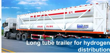
Long tube trailer for hydrogen distribution
