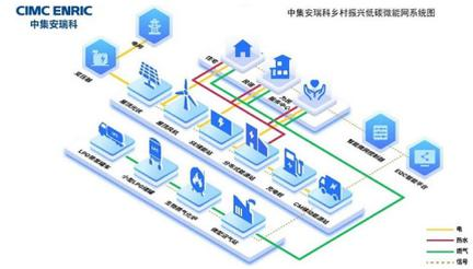
Low-carbon Micro Energy Network System Diagram of CIMC Enric for Rural Revitalization
