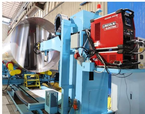
Anti-wave Plate TIG Automatic Welding Robot Workstation
