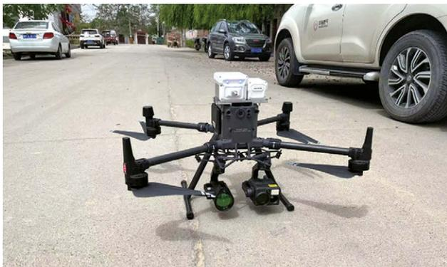
Unmanned Natural Gas Leakage Patrolling Detection System
