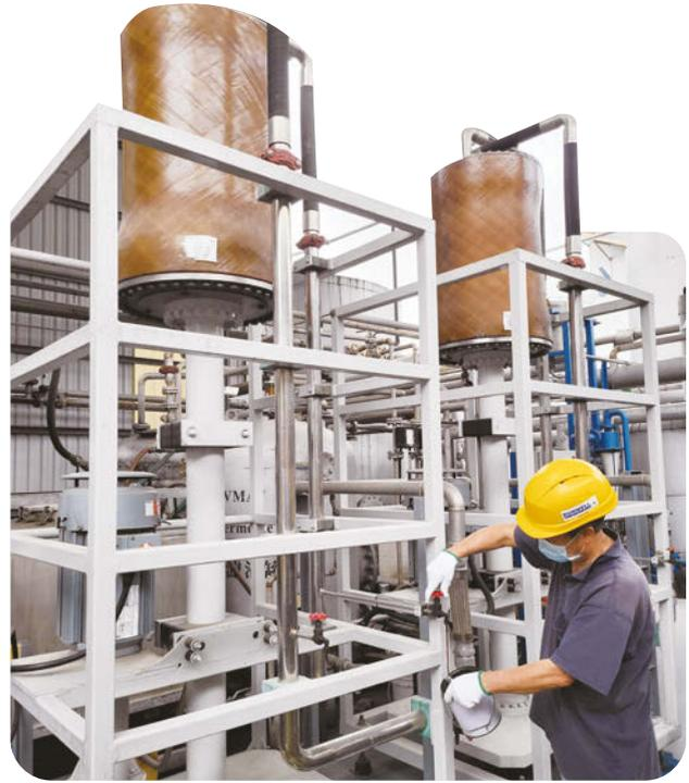
● Waste oil recycling using VMAT technology
