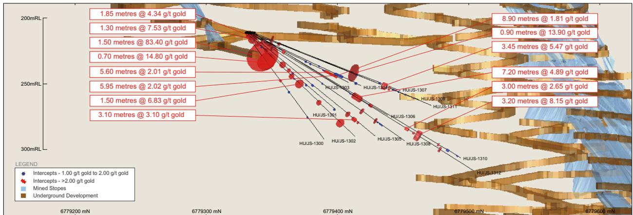
**Figure 5 – Arpola-3 2023 Drill Hole Vertical Section. View looking west.**
