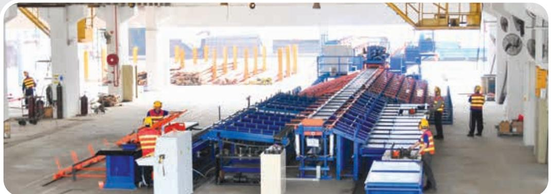
Automated Cut-and-bend Rebars Processing Plant in Tai Po, Hong Kong
