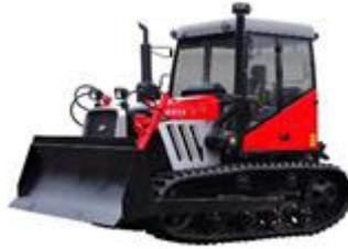
The walking device is a crawler type, mainly used for pulling and driving various supporting equipment, agricultural machinery for completing agricultural operations, various earthwork operations, transportation operations and fixing operations.
