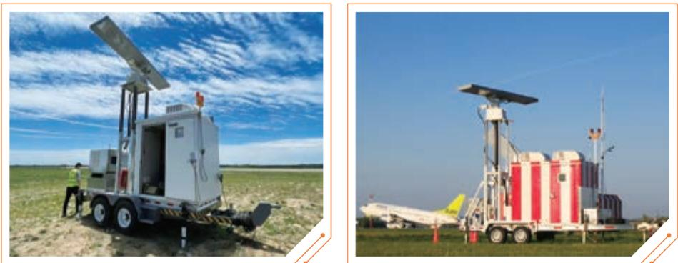
Figure 4: Warning Radar for Bird Strike Prevention
