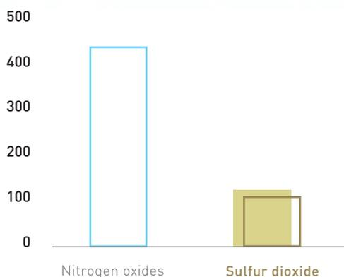
According to the standards set by the local environmental protection bureau for waste emissions, the annual limit of nitrogen oxides are 549.25 tons, and the annual limit of sulfur oxides are 327.1 tons. As shown in the above figures, the NO<sub>x</sub> and SO<sub>x</sub> emissions of the Group in 2021 were 431.73 tons and 104.47 tons respectively. The total emissions of the two major air pollutants have not exceeded the standard indicator.
