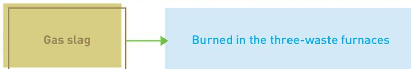
Unlike urea producers who use natural gas as raw materials, we use coal for urea production, so a large amount of waste residue will be generated during the production process. We send the generated waste slag to three waste furnaces for combustion. After combustion, some waste slag can be recycled as boiler fuel, and some waste slag can be processed into new building materials and sold to other companies.
