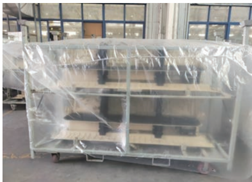
Before the change – with disposable bagging tooling 變更前—帶一次性套袋工裝
