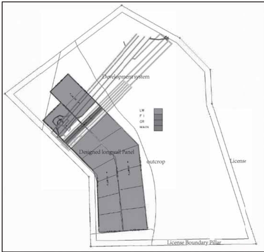
Figure 9-2: Mine Design and Longwall Panel Layout (Seam No.6-1 in first mining district)
