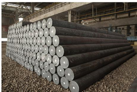
Pipe billets are made from scrap metal. They are a cylindrical material that meets the requirements of other oil pipes and energy equipment manufacturing. Pipe billets, through further processing, may be made into other oil pipes and energy equipment materials of different specifications for different purposes. Pipe billets manufactured by us are either further processed by us for the production of other oil pipes or sold to our customers in the PRC.
